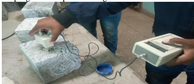
Figure 7. Electrical Resistivity Test in Progress
