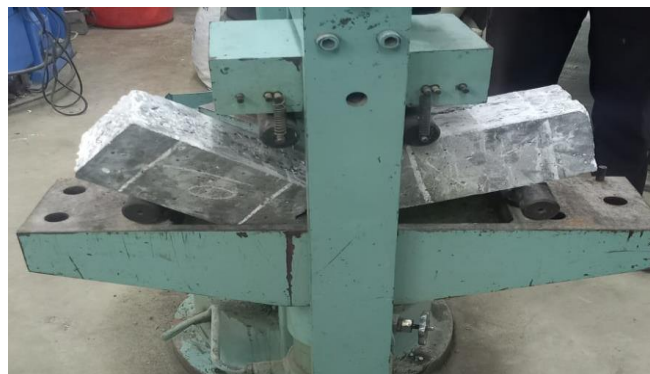
Figure 9. Beam Failure under Flexural Load
