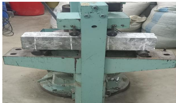
Figure 6. A Beam on the Flexural Testing Machine
