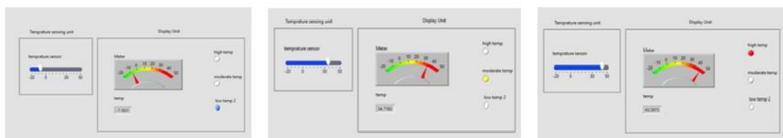
Figure 6. LabVIEW program that for low, moderate and high control of temperature
