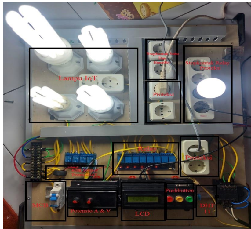
Figure 3. Electrical Protection and Monitoring Automation Tools
