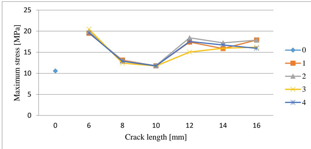
**Figure 10.** The maximum stress of the overhung rotor with a crack between the two supports
