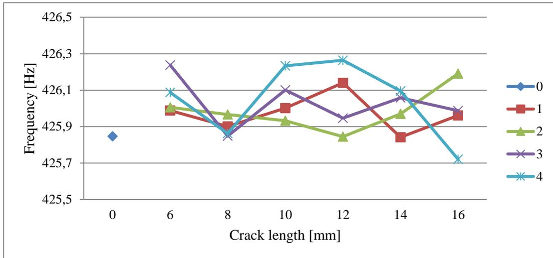
**Figure 5.** The third natural frequency of the rotor due to crack length for various crack depth with the location of the longitudinal crack between disk dan bearing
