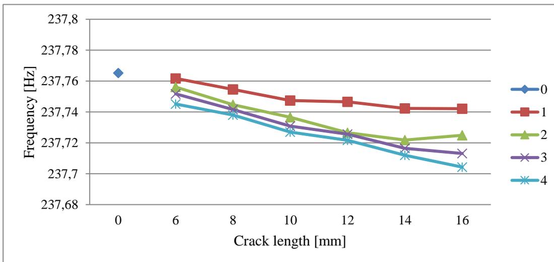
**Figure 4.** The second natural frequency of the rotor due to crack length for various crack depth with the location of the longitudinal crack between disk dan bearing
