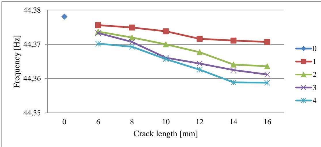
**Figure 3.** The first natural frequency of the rotor due to crack length for various crack depth with the location of the longitudinal crack between disk dan bearing
