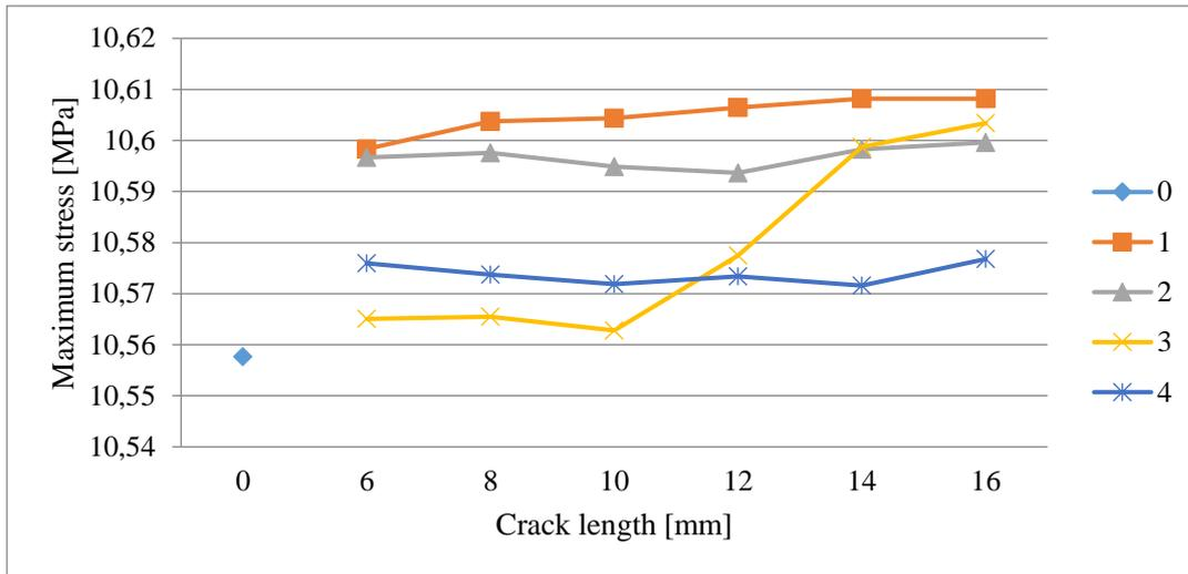
**Figure 9.** The maximum stress of the overhung rotor with a crack between disk and bearing
