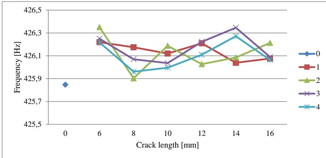
**Figure 8.** The third natural frequency of the rotor due to crack length for various crack depth with the location of the longitudinal crack between two supports
