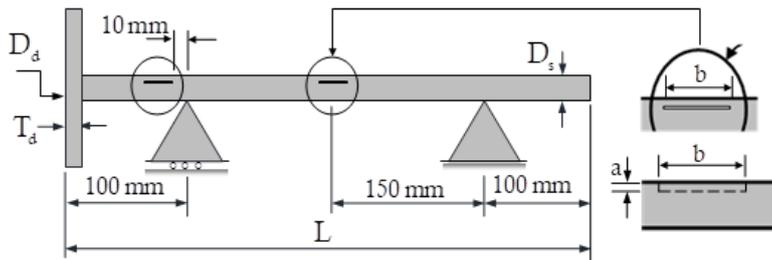
**Figure 1.** Overhung rotor system with longitudinal crack
