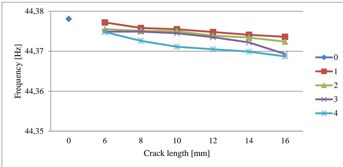
**Figure 6.** The first natural frequency of the rotor due to crack length for various crack depth with the location of the longitudinal crack between two supports
