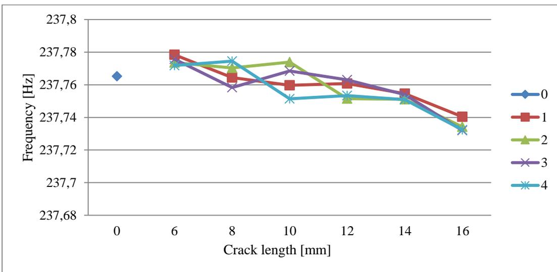
**Figure 7.** The second natural frequency of the rotor due to crack length for various crack depth with the location of the longitudinal crack between two supports
