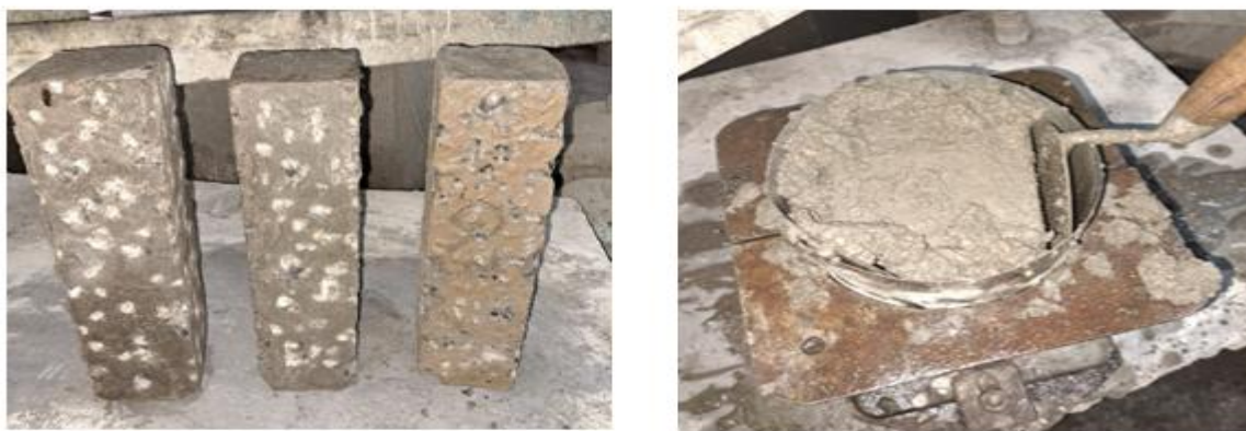
Figure 2. Specimen circularisation process: (a) roughened specimen and (b) mortar placement around the specimen
