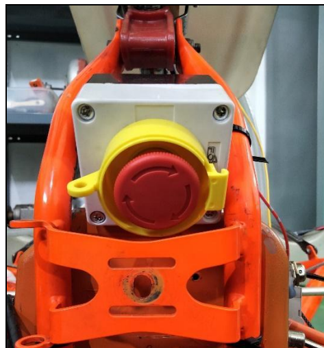
Figure 7. Emergency Stop Switch
