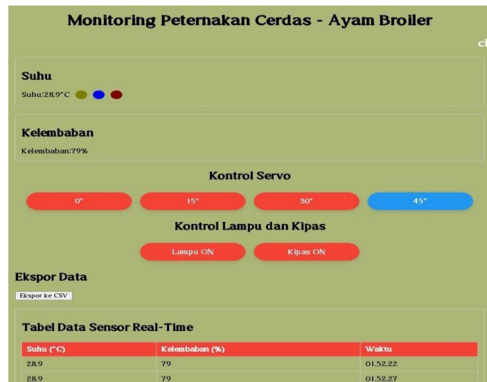
Figure 15. Controlling the servo angle for feeding
