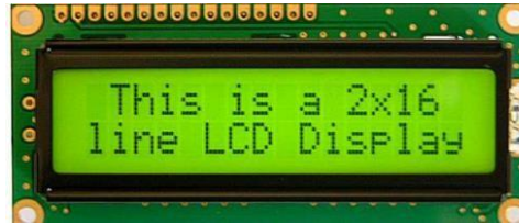
Figure 2. The 16x2 LCD
