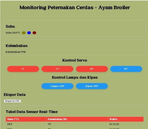
Figure 17. Control buttons for lights and DC fan
