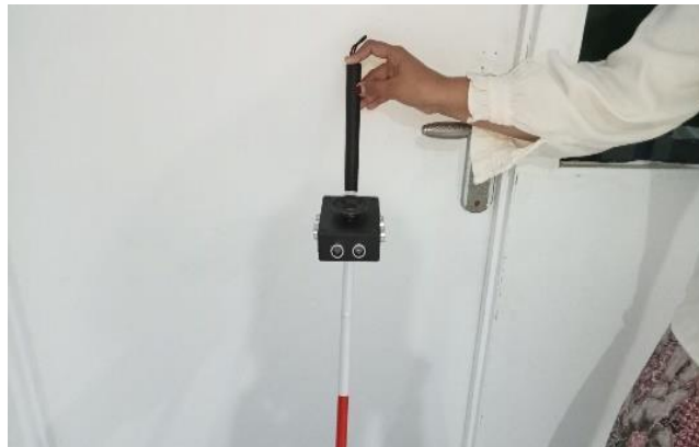
Figure 6. Tool Installation on the Stick
